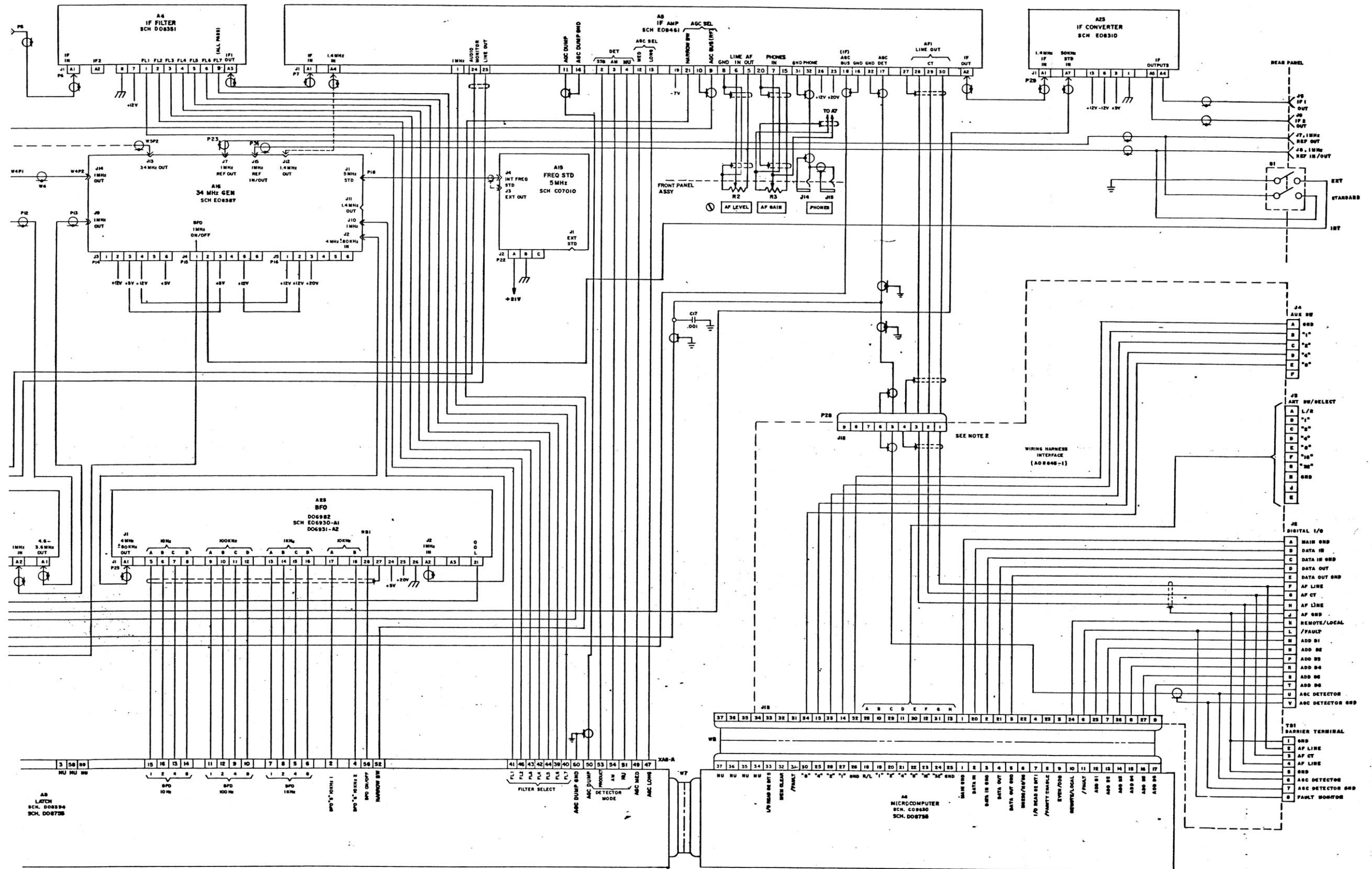
Figure 5-6 RA6778C LF/HF Radio Receiver, Chassis Wiring Diagram (Sheet 2 of 3)
