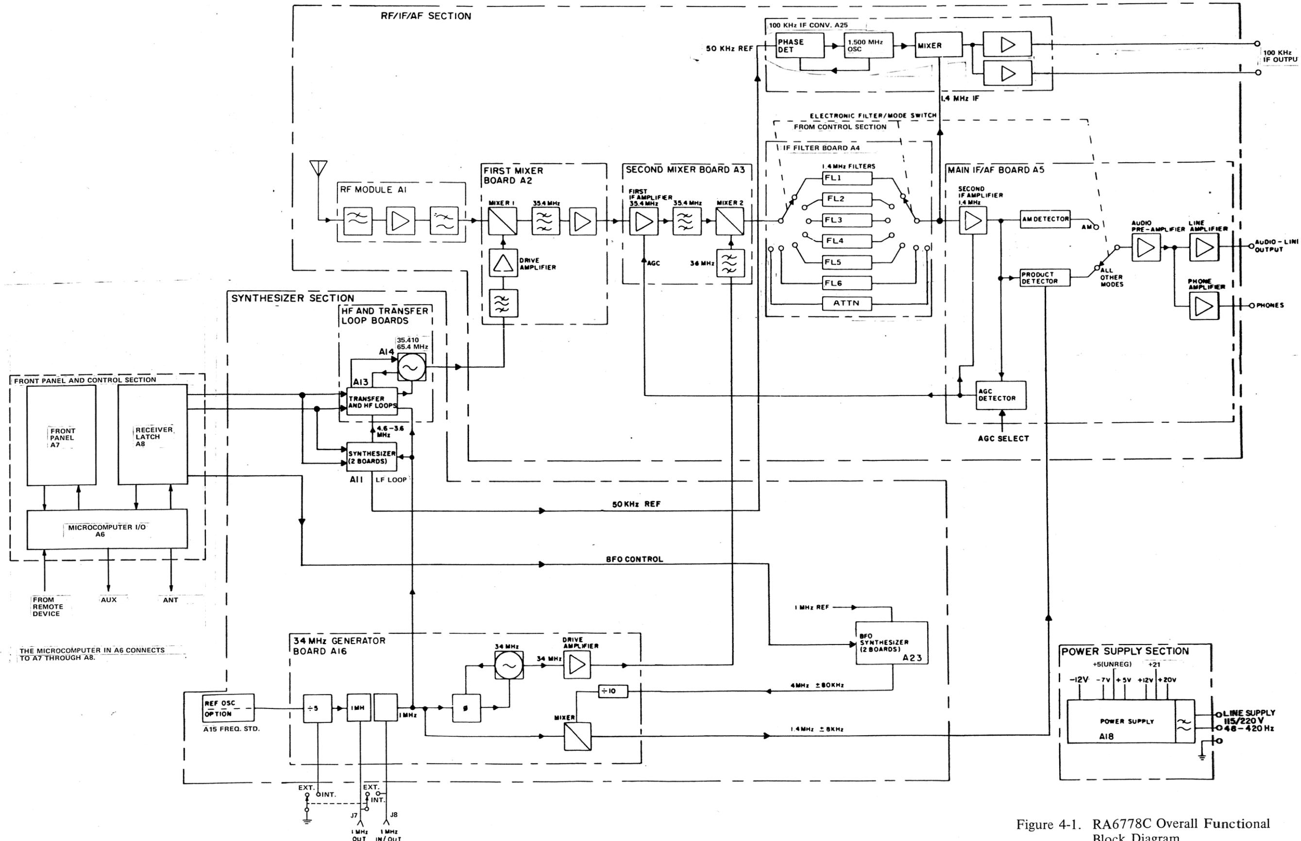
Figure 4-1. RA6778C Overall Functional Block Diagram
