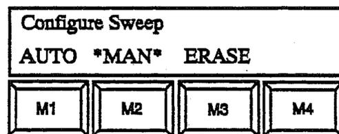
**M1:** To configure Auto sweep operation. In this mode the step size is always set to set to half the receiver bandwidth (i.e. changes when the bandwidth does), and the subsequent menus allow the average sweep dwell time and COR action to be set up.
