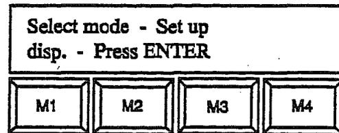
The display then returns to the mode/bandwidth/AGC/BFO display to enable the desired preset parameters to be entered. This time however, the mode must be defined by pressing the desired mode pushbutton. The remainder of the procedure is as before.
