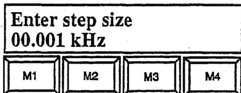
following menu is presented to allow a step size of between 1 Hz and 99.999 kHz to be selected.
