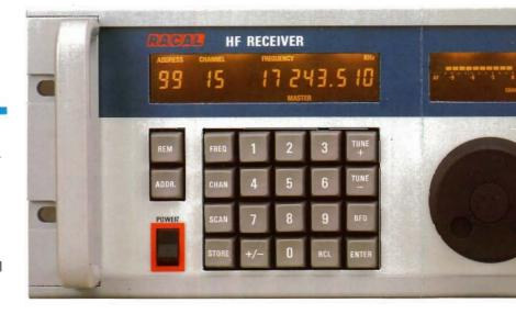
BFO – Enables the BFO frequency to be set in CW mode, either using the main tuning knob or the +/– key and numeric keys.
